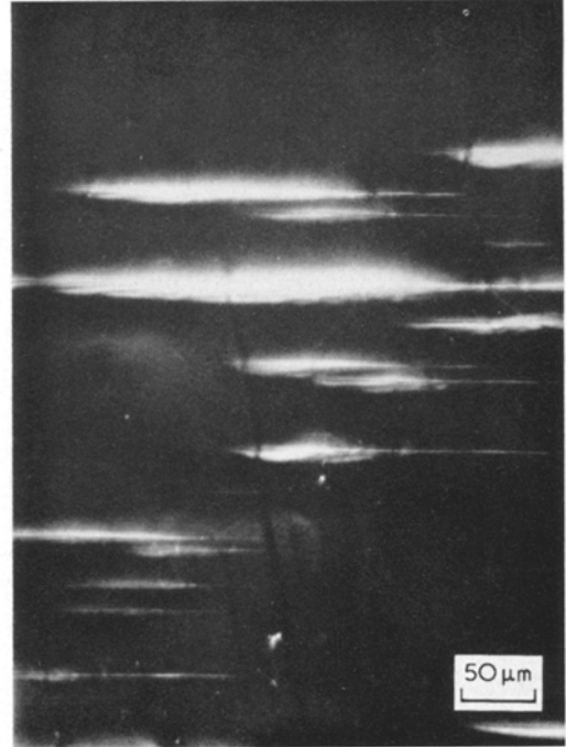
Figure 5 Shear crazes in 2:1 drawn PET for \theta = 90^\circ .
